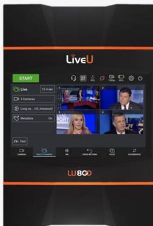
The LiveU encoders uses cellular bonding technology (LRT) that adds multiple cellular networks together to create redundancy and reliability to the video encoding.
