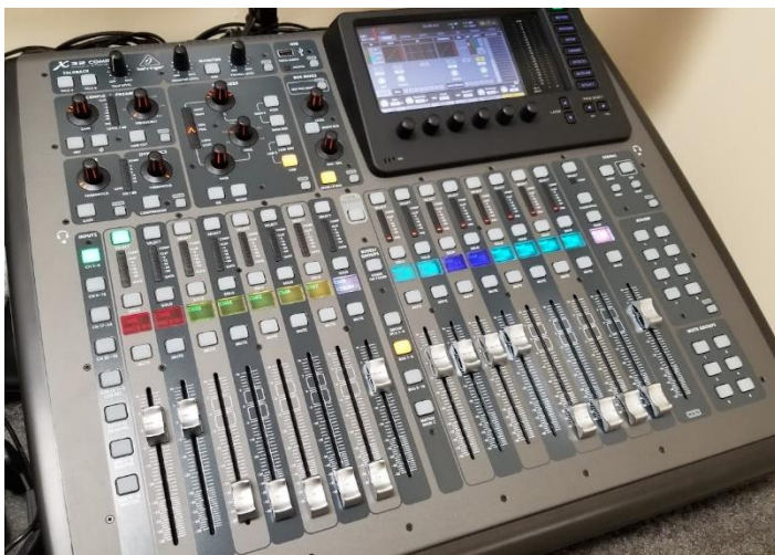
X32 Compact w/ Dante Expansion - Supports 64 Channels of Dante 32in/32out (Varto Technologies, East Rutherford, NJ)
