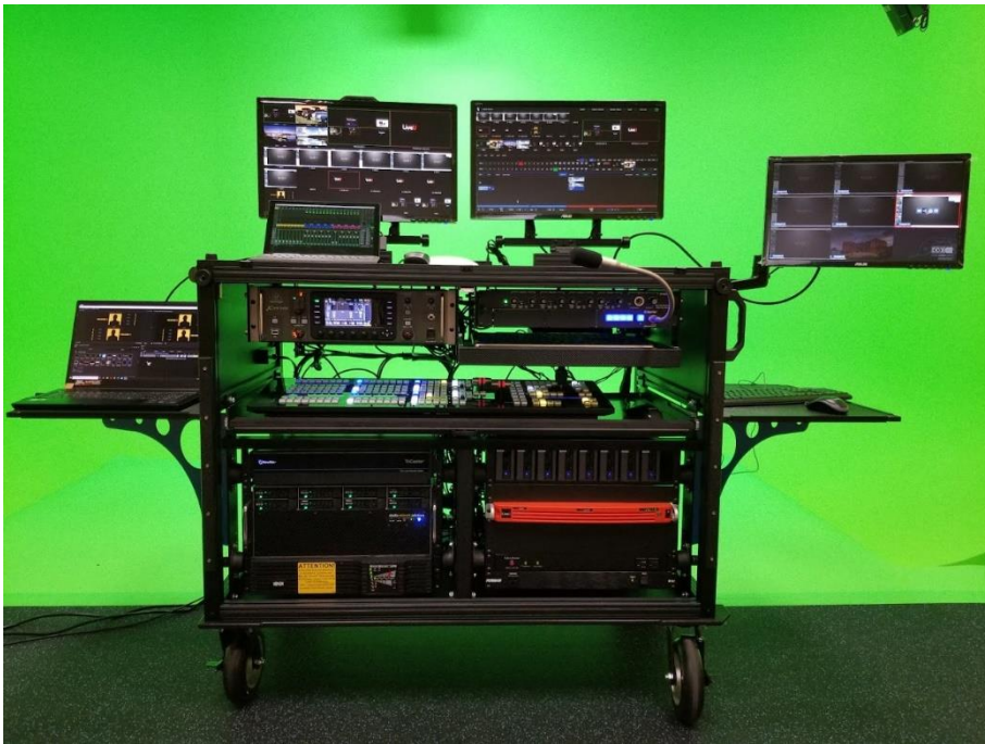
Mobile REMI Production Cart (Includes TriCaster, LiveU, 8 Zoom PCs, Dante Audio Mixer, 48TB Network Storage Solution & More! (Varto Technologies, East Rutherford, NJ)
